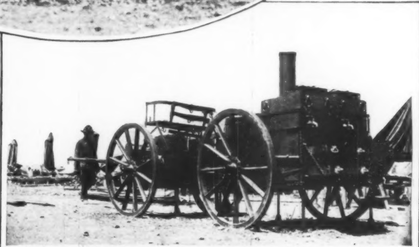
FIELD KITCHEN ON THE MARCH These field kitchens are drawn by horses or mules, and keep cooking while en route, so it is always possible to have hot meals ready on time. The guard is not fully equipped with these kitchens, but those in use are so successful that every company should eventually have one.
